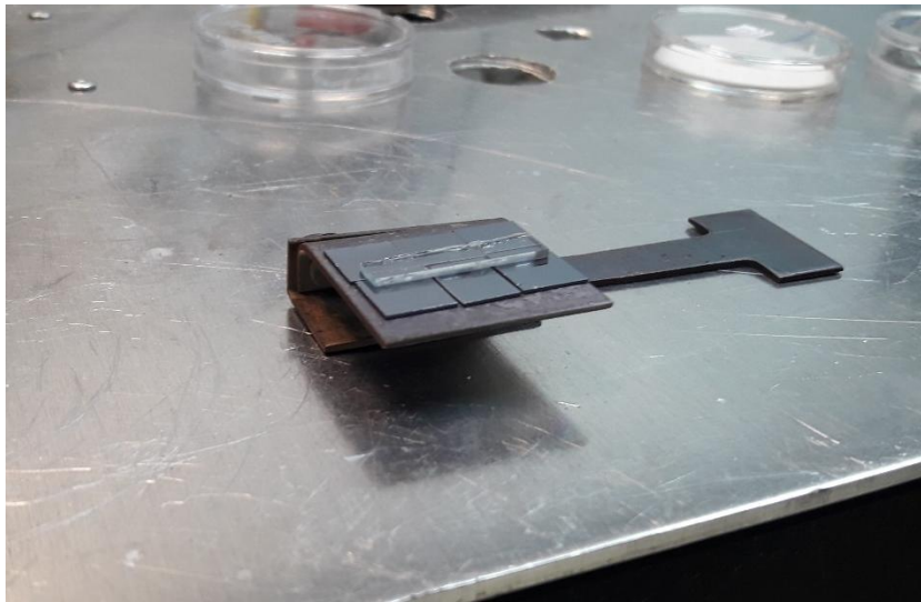
Figure 10. Si (001) substrates ready to be introduced in the sputtering equipment
